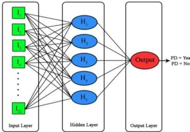
Fig. 3. Multilayer Perceptron Structure [3]
