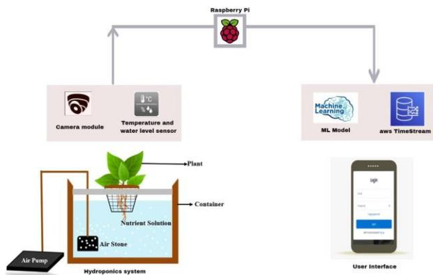
Fig. 1: Architecture of Hydroponics System
