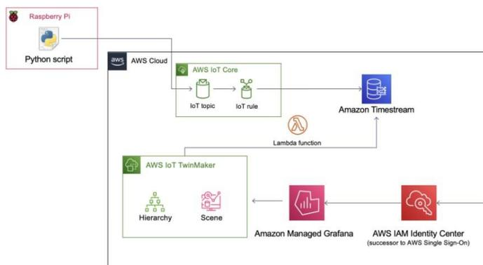
Fig. 3: Architecture of AWS TwinMaker
