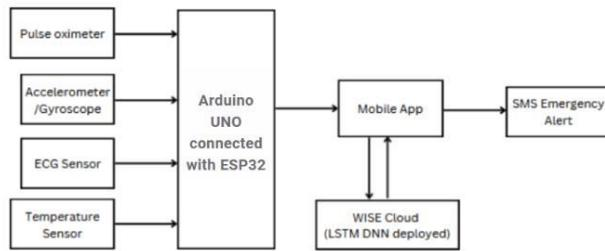
Fig. 1. Block Diagram of the proposed system.
