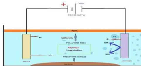
Fig 1 Schematic representation of the electrocoagulation cell.
