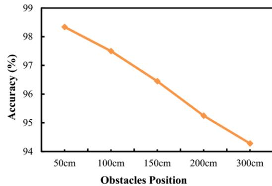
Fig. 2. The Ultrasonic sensor accuracy graph
