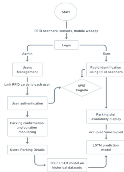
Fig 3.1 System Process Flow
