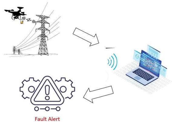
Fig.1. Block diagram of Proposed system- fault detection of power transmission lines using UAV
