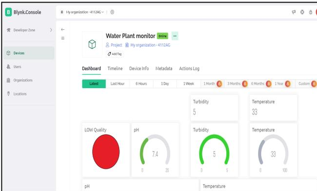
Fig 8: Levels of current water pH count, water temperature and Turbidity of impure water.
