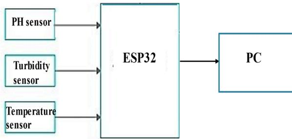
Fig 1: Block diagram of water quality monitoring system
