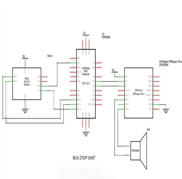
Fig. 2. Circuit diagram of the Bus Stop Module.
