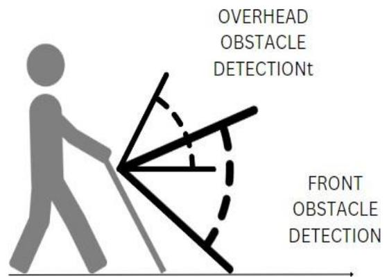
Fig. 5. Image detection angles of the blind stick module.
