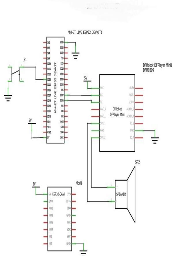
Fig. 1. Circuit diagram of the Blind Stick Module.
