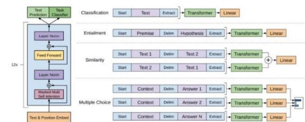
(left) Transformer architecture and training objectives used in this work. (right) Input transformations for fine-tuning on different tasks. We convert all structured inputs into token sequences to be processed by our pre-trained model, followed by a linear+softmax layer.
