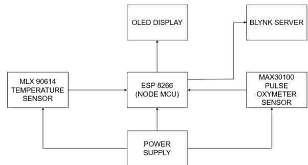
Fig. 2. Block Diagram for Biotelemetry
