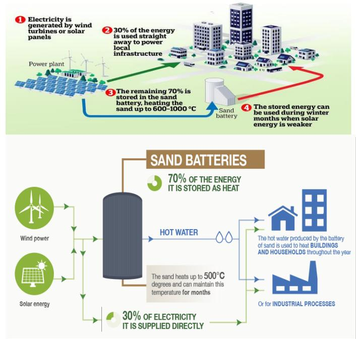
Fig1: Working of sand battery
