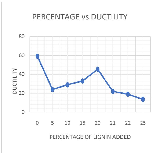
Figure 3: Graphical representation of percentage of lignin added Vs ductility values obtained.
