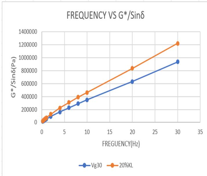
Figure 5: Graphical representation of frequency Vs  $G^*/\sin \delta$  of Vg30 and 20% LBC binder
