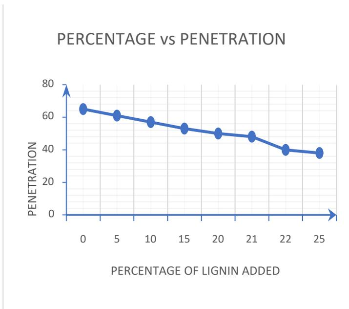
Figure 1: Graphical representation of percentage of lignin replaced Vs Penetration Value
