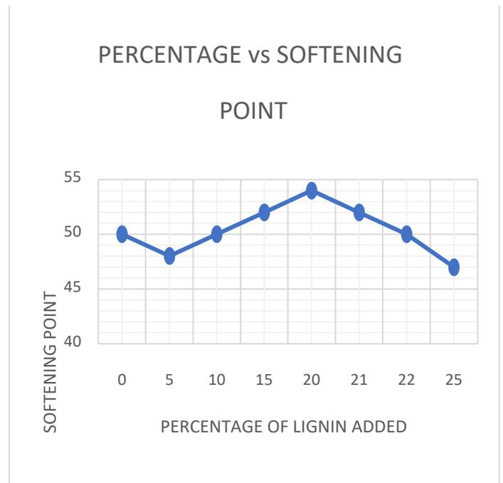
Figure 2: Graphical representation of percentage of lignin added Vs softening point values
