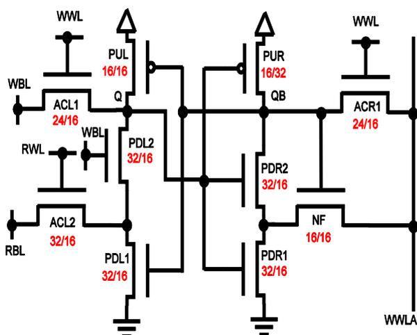
Fig. 4. Proposed High Speed Low Power 10TSRAM(HS10T)
