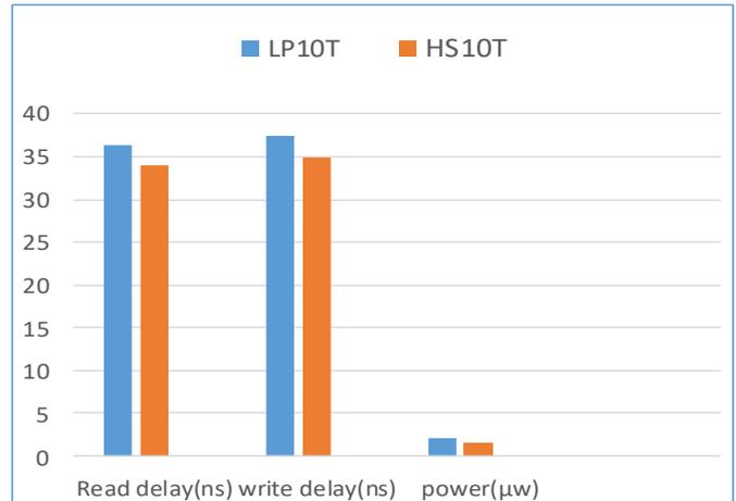
Fig. 7 Comparison in terms of delay and power.
